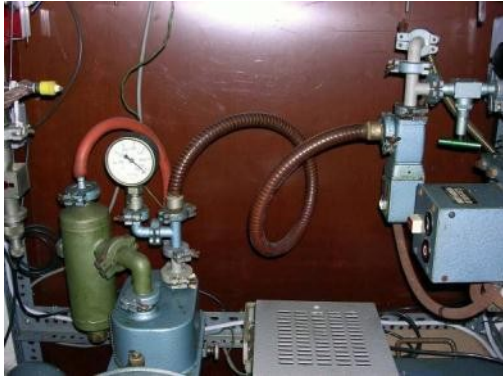
26 Connection of rotating pump and diffusion pump
