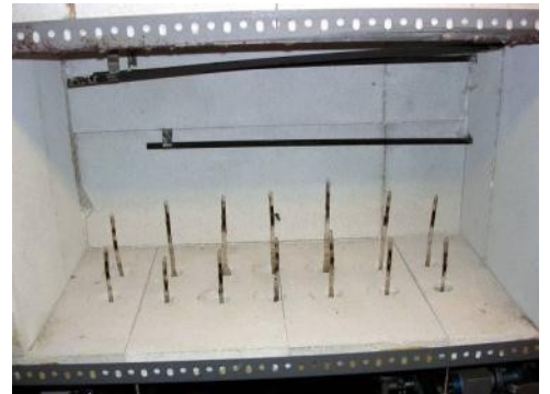
28 View into the pumping oven
