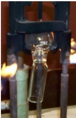
22 The glass softens and melts tight to the disk
