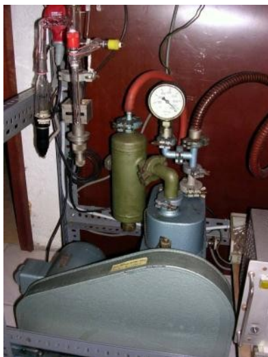
23 Two step rotating pump
